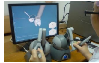
Figure 1 A dentist performing access opening to the root canals with a haptic virtual reality simulator
